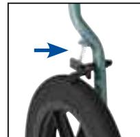
Alternatively, the user or attendant may lock the brake using the lower brake lever on the self propelled wheel. Simply push the lever forward to lock and pull back to release.
